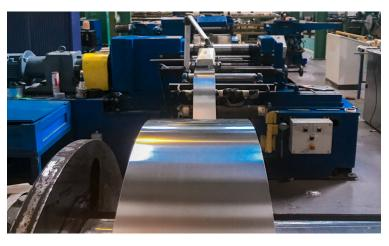
Low Width Thickness Ratio 3:1 unique to the industry (normal minimum is 8:1)
